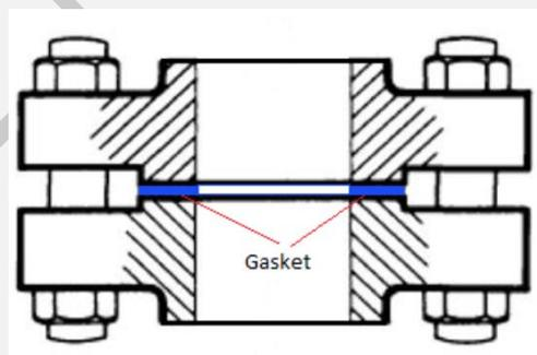
The typical flange face finish for ASME B16.5 RF flanges is 125 to 250  $\mu\text{m Ra}$  (3 to 6  $\mu\text{m Ra}$ ).
