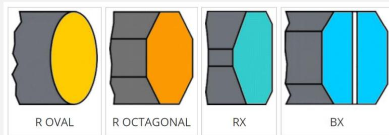
The RX type is suitable for pressures up to 700 bar. RTJ is capable of sealing itself. The outer sealing surfaces make the first contact with the flanges. A higher system pressure causes a higher surface pressure. Type RX is interchangeable with the standard R-models.
