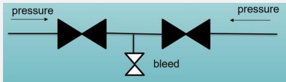
The bleeding connection is done between the two valves, which can be integrated in one body.
