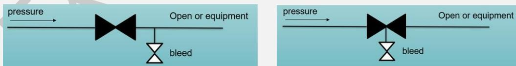
The sealing of the valve is only reached when the flow is always in the same direction.
